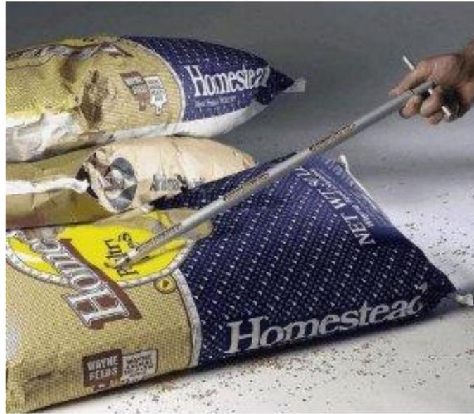
Figure 3 Sampling probe in use
